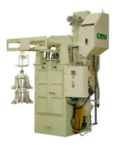
**Motorized hangers:** the movement of the hangers has been motorized. Now the system moves the hook inside of the blasting chamber at the beginning of the operation and removes it at the end of the blasting. The actuation of this system is performed by the operator through the control panel. **Simple like that.**
